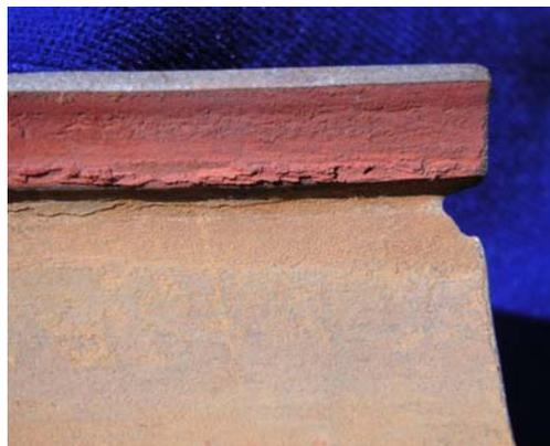
**Figs. 5 + 6** Carbonic acid corrosion on condensate return tube (right = enlargement)
