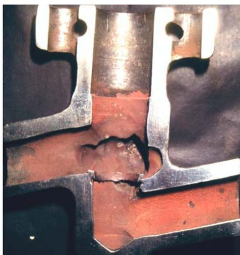
**Fig. 7** Erosion corrosion on a steam block valve used as control valve
