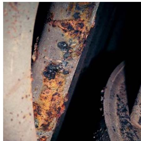
**Fig. 4** Oxygen corrosion on smoke tube
