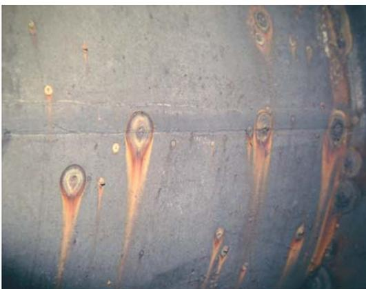
**Fig. 3** Oxygen corrosion on fire tube of a horizontal shell boiler
